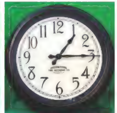
■ PHOTO 4. Impulse secondary from engineering dept.; soft copper shell and painted face.
